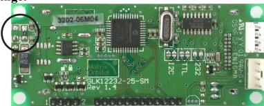
Here is the <u>current</u> backlight resistor values for the following displays: GLK12232-25-SM PCB Rev 1.4 (-GW and -WB): 75 Ohms GLK12232-25-SM-V PCB Rev 1.4 (-GW and -WB): 61.9 Ohms
