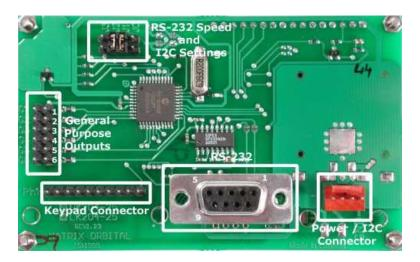
Figure 2: Electrical Connections
