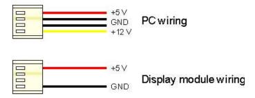
Figure 4: Wiring for 5V Modules
