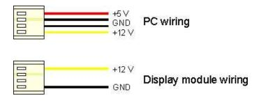
Figure 6: Wiring for 12V Modules
