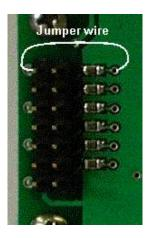
Figure 11: Bypassing 240 ohm Resistor
