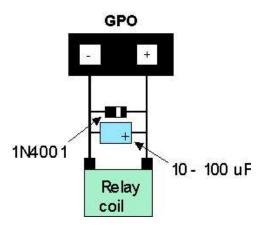
Figure 12: Clamping a Relay
