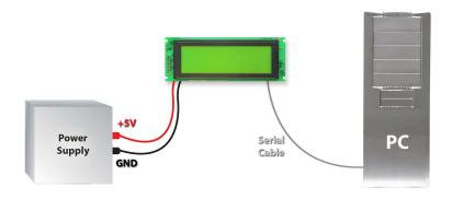
**WARNING** DO NOT use the standard floppy drive power connector, as this will not provide you with the correct voltage and will damage the display module.
