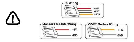
Figure 6: PC vs Matrix Orbital Display Module Wiring
