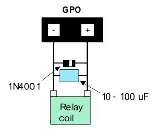
Figure 2-10 Clamping a Relay
