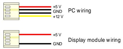
Figure 2-3 Power Connector wiring differences
