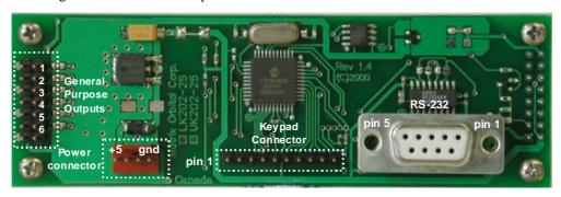
Figure 2-1 Electrical Connections
