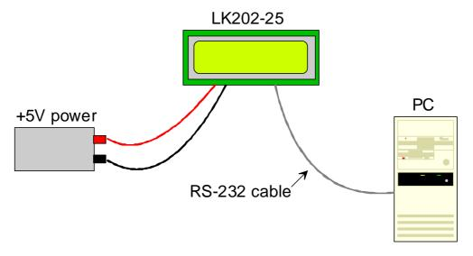
Figure 1-1 Connections for Testing
