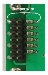
Figure 2-9 Bypassing 240 ohm resistor
