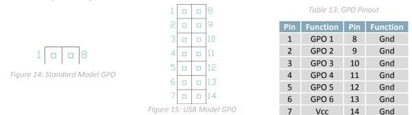
A unique feature of the GLK24064-16-1U is the ability to control relays\*\* and other external devices using either one or six General Purpose Outputs. Each can source up to 10mA of current at five volts when on or sink 20mA at zero volts when off. The two row, fourteen pin header can be interfaced to a number of female connectors to provide control to any peripheral devices required.
