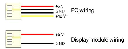
Figure 2-3 Power Connector wiring differences
