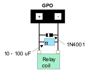
Figure 2-11 Clamping a Relay
