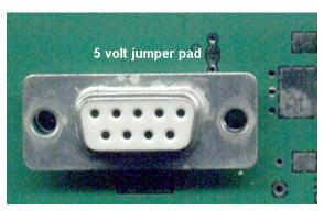
To use pin 9 as the power source, the user must solder the 5 volt jumper pad beside the DB9 connector. If you have any further questions or concerns don't hesitate to contact Matrix Orbital at support@matrix-orbital.com.
