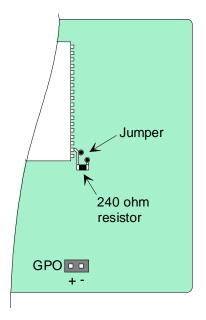
Figure 2-10 Bypassing 240 ohm resistor
