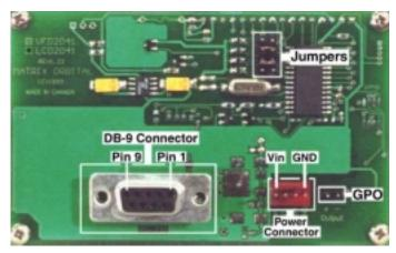
Figure 2-1 Electrical Connections
