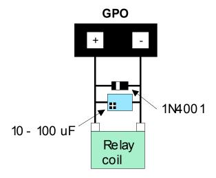
Figure 2-11 Clamping a Relay
