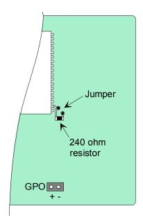
Figure 2-10 Bypassing 240 ohm resistor
