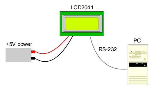
Figure 1-1 Connections for Testing
