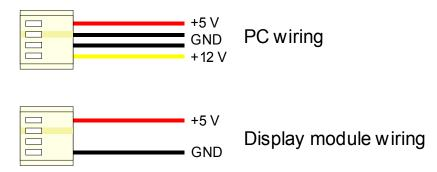
Figure 2-3 Power Connector wiring differences
