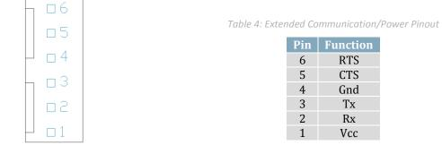
Figure 9: Extended Communication/Power Header
