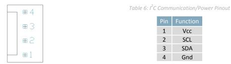
*Figure 11: I<sup>2</sup>C Communication/Power Header*
